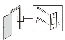
With the door closed, use a flathead screwdriver to test if deadbolt works smoothly.
