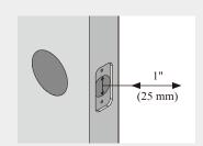
Measure to confirm that the door is 1-3/8" to 2" (35 mm or 50 mm)thick
