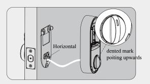
D Test operation using backup key and thumbturn for smooth rotation.
