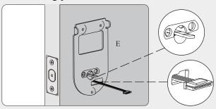
D Secure the mounting plate with the screws J. Do not overtighten screws.
