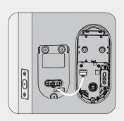
C Rotate the thumbturn and keep it poiting upwards. Make sure the latch is still fully retracted (unlocked).
