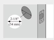
В Measure to confirm that the backset is either 2-3/8" or 2-3/4" (60 or 70 mm)
