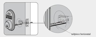
C Send the cable through the bottom horizontal slot in the mounting plate.
