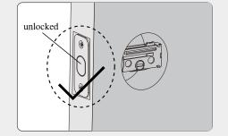
Route the cable below the latch and insert the cylinder tailpiece through the horizontal slot in the latch.
