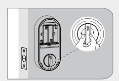
E Secure the interior assembly with screws K.
